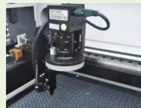
Optional:Camera pick up positioning, San the material,cutting more efficient and precision
