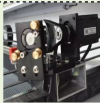
Reflect 45° mirror adjustment set.Three -point dimming bolt for easier dimming
