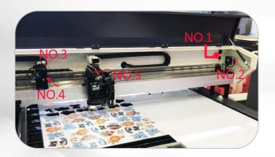
4. Constant light path Patent design), composed of five reflective mirrors: the distance between laser beam output to the focus head is always the same, whatever the machine move. More advanced than common light path composed of 3 mirrors or fake 5 mirror light path.
